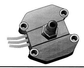
The OMEGA®PX240APressure Transducer Series is available in gage type to measure pressures ranging from +/- 2.5 psi to 0-250 psi. The sensor is housed in a rugged stainless steel body. Media compatibility for oils, fuels, gasoline, petroleum-based lubricants, hydraulic fluids, alcohol, water and air is provided by internal Buna-N O-ring seals. Termination is by 300mm (12 in.), colour coded 18 gage lead wires
