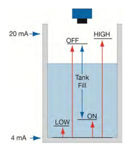
• Lo Alarms (Lo) – Used to energize a relay (ON) when the level falls below the Lo setting. Relay will de-energize (OFF) when level rises above the original setting.
