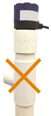
Avoid the use of a tee within the stand pipe. A tee can create false signals impeding the sensor's performance.
