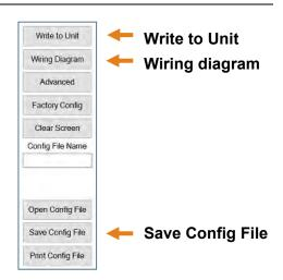
"Save Config File" will save this configuration as a text file which can be loaded back into LVCN414-SW by pressing the "Open Config File" button. It is good practice to save the configuration file for each different configuration with a unique name for easy identification. If using multiple sensors in identical applications, then use of a single configuration file is recommended.
