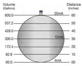
**Note:** In the above illustration, 1" of liquid does not equal 10 gallons. The 10" at the bottom represents a rise of 62.8 gallons. As a change between 10" and 20" represents an increase of 109.6 gallons (i.e. 172.4 gallons – 62.8 gallons).
