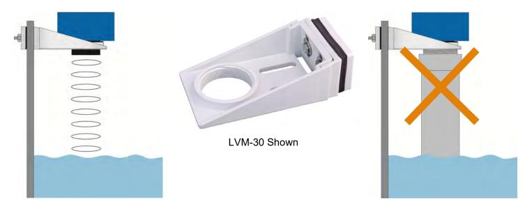
**Note:** The Side Mount Bracket (LVM-30 series) is not designed for use with stand pipes or as a method to secure stand pipes. There are too few threads to properly hold the sensor and the stand pipe.
