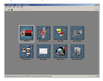
The software is designed such that the first three icons are the only ones required for the majority of simple applications. The remainder of the icons provide access to the Master's more advanced features, such as programming, data logging and the web server.
