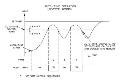
As shown above, the setpoint used during auto-tune is the value 75 % above the difference between the current PV and the setpoint. This allows the oscillations to occur close to setpoint, while avoiding excessive overshoot. Since the module performs on/off control during auto-tune, it is important to set a suitable On/Off Hysteresis value prior to invoking auto-tune.
