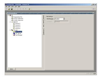
The properties on the General tab are used to enable or disable the mail manager, and to provide a name for the Master. This name will be used within email messages to identify the originator of the message. Applications will typically use the name of the machine to which the Master is installed, or the name of the site that it is monitoring.
