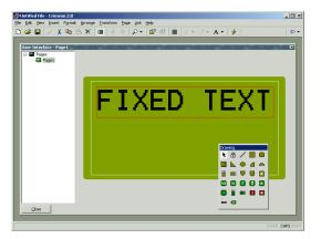
Only the US English text can be edited directly. The international versions of the text must be edited via the properties dialog box, which is accessed by selecting the primitive and pressing **Alt+Enter**, or by selecting the Properties command from the Edit menu...
