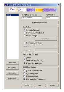
You will now be able to configure any Windows-based software to use the newly-created COM port for download. When the software opens the connection, the Master will suspend communications on the shared port, and then data will be exchanged between the PC software and the remote PLC—just as if they were connected directly! When the port is closed, or if no data is transferred for a minute, communications will be resumed.
