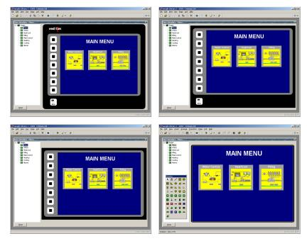
As you can see, at each level, fewer keys are shown, and more of the window is allocated to the display itself. The panel view level can be controlled from the View > Panel menu, or by using the panel icon  $\square$ , or by pressing the **Alt** key together with the digits 1 through 4.
