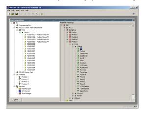
To indicate that you want a particular register within your gateway block to correspond to a particular data item, simply drag that item from the right-hand pane to the left-hand pane, dropping it on the appropriate gateway block entry. The example above shows the PV variables of four PID modules mapped to PLC registers N010:0000 through N010:0003.
