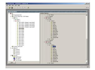
Certain module data are read/write variables, allowing them to be controlled by the PLC or HMI to which the MC is connected. To map writeable variables, follow the same procedure as shown above, but this time, set the Direction property to Device to MC. Note that with the Direction property set for Device to MC, only writable variables will appear in the right pane.
