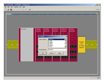
Edit the individual module's properties by double-clicking it. Each module and its properties are explained in detail in later sections.
