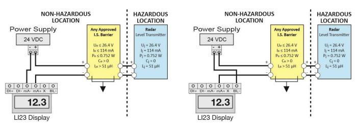
**Note:** Always refer to the Control Drawing 301901 for further wiring information.
