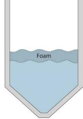
**Light Foam** – If foam partially covers the surface of the liquid, set Foam to No.
