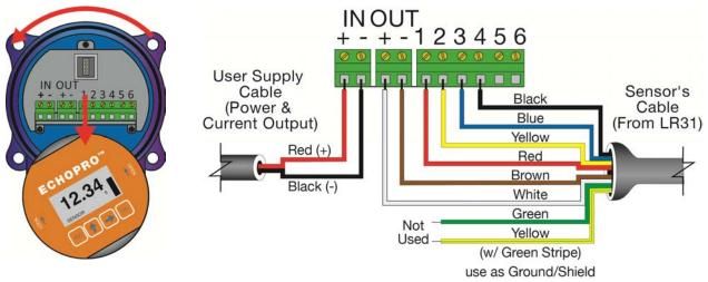
The attached 8-conductor sensor cable (only 6-wires are used) will wire directly into the display terminals. A shielded 2-wire cable (user supplied) is required to provide power to and the current output signal from the display. To confirm the 4-20mA output, place a multimeter (VOM) set to read milliamps in series with the (-) wire (see below).
