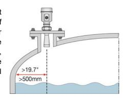
Avoid mounting the sensor in the center of a dome top tank. The center of such a tank will multiply the echoes, making sensor operation difficult.
