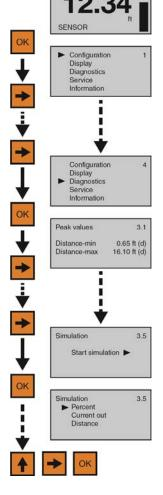
This method uses distance from the sensor's measurement location to set the current output (4-20mA) between the Empty and Full Configuration values.
