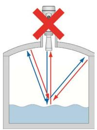
In cone bottom tanks, it can be advantageous to mount the sensor in the center of the tank, making it possible for the sensor to measure closer to the bottom of the tank. If the sensor is mounted over an angled bottom, and the level drops below the angle, the echo will be deflected away from the sensor, resulting in poor operation. The sensor can be mounted over an angled bottom as long as the level is maintained within the straight side wall so the sensor will receive echo returns.
