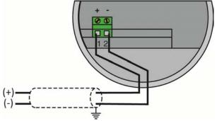
The sensor should be wired with shielded 2-conductor cable (16 to 22 AWG) to protect from electromagnetic interference. If using a liquid tight connector, select a cable with an outer diameter that is designed to ensure an effective seal with the connector [typically between 0.20" to 0.35" (5 to 9 mm)].
