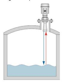
**←←←** Correct Mounting **←←←** Sensor mounted off center in a dome top tank.
