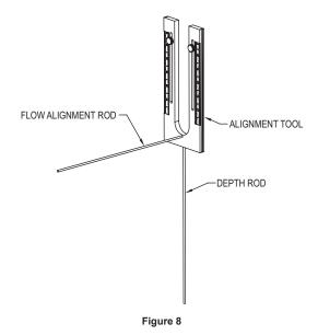
3. Rotate the transmitter so the pipe alignment rod is parallel with the flow in the pipe.
