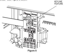
7. Plug the other end of the cable into the bottom of the supplied portable display being sure to orient the keying feature/tab as shown:
