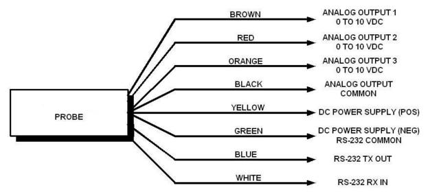
Figure 3-3a HX80A Series Probe (with Discrete Wires) Wiring Diagram
