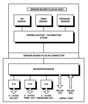
Figure 4-1 Basic Block Diagram, Probe Assy
