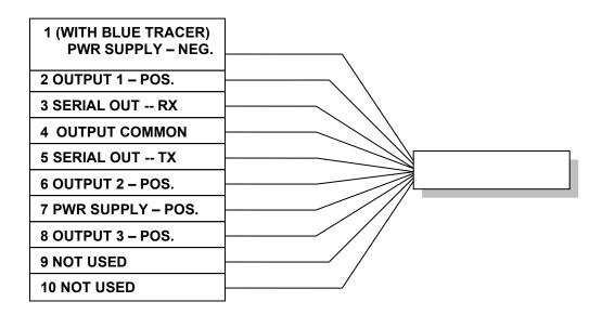
Figure 3-3 HX80A Series Probe (with Ribbon Cable) Wiring Diagram
