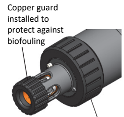
Make sure the closure cap is installed before deploying the logger
