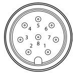
Figure 14: Female Mating M12 8-Pin Connector
