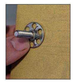
Figure 7: Sand the adhesive studs
