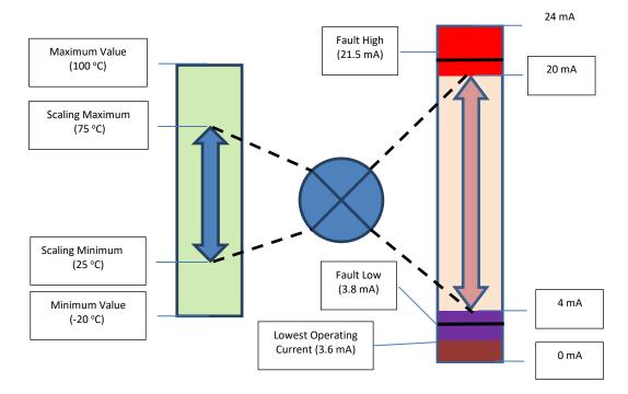
Figure 26: SYNC Configuration Software – Sensor Mapping
