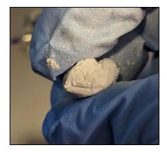
Figure 9: Thoroughly mix the epoxy
