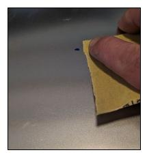
Figure 6: Clean and sand the surface the device will be mounted on
