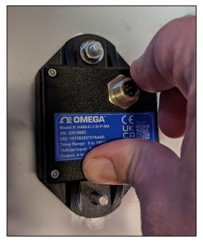
Figure 13: Secure the hardware nuts to properly mount the HANI™ Tank Sensor
