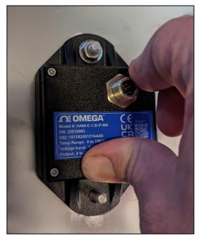
Figure 4: Secure the hardware nuts to properly mount the HANI™ Tank Sensor
