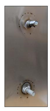
Figure 3: Included studs welded to tank
