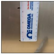
Figure 5: Measure out mounting stud points at 3.5"
