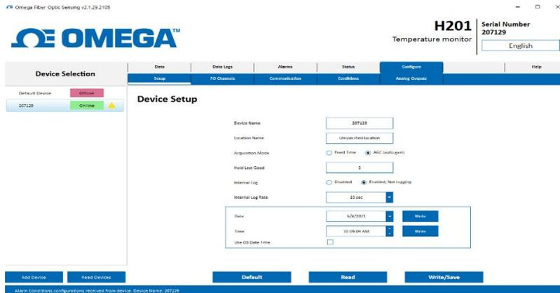
After a few seconds, this Configuration window is populated, and you can change any parameters you want (some fields, in light grey, are for information only and are not changeable); do not forget to click the “Write/Save”, button, to save your new parameters to the instrument.
