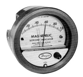
The Dwyer Series 2000SP Magnehelic® gage/setpoint indicator combines an analog differential pressure gage with a red LED to indicate when pressure reaches a field adjustable setting. The black pointer continually indicates applied pressure while the externally adjustable red pointer shows the pressure at which the indicating LED on the right side of the scale will illuminate.
