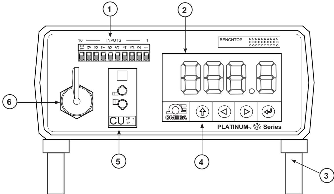
**Figure 2. MDS8PT Front Panel. (Not to scale)**
