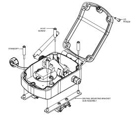
**DIN Rail Mounting Bracket Installation**
