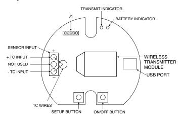
Main Transmitter Board/Input Connections
