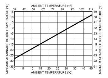
The Effect of Increased Ambient Temperature on Operating Temperature
