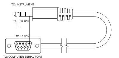
Connecting the CL1500 to a Computer's Serial Port
