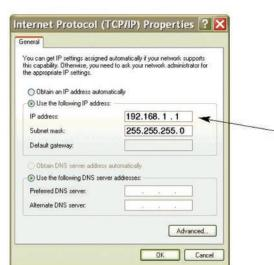
You can access the Coordinator's web server via any internet browser using IP address of **192.168.1.200**. Once you log into the Coordinator's web server, you will be able to change its IP configuration according to Section 4.2.
