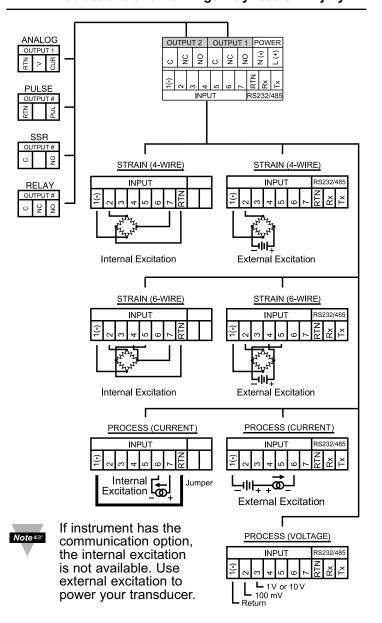
Connect the main power connections in the figure shown below.
