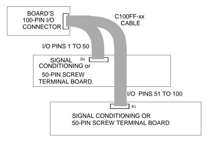
Figure 3-2. Cable C100FF-xx Configuration
