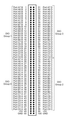
Figure 3-1. PCI-DIO96 100-Pin Connector Pin Out
