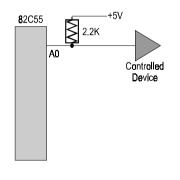
Figure 7-1. Pull-up Resistor
