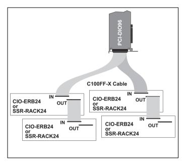
Figure 3-4. Relay Rack Cabling
