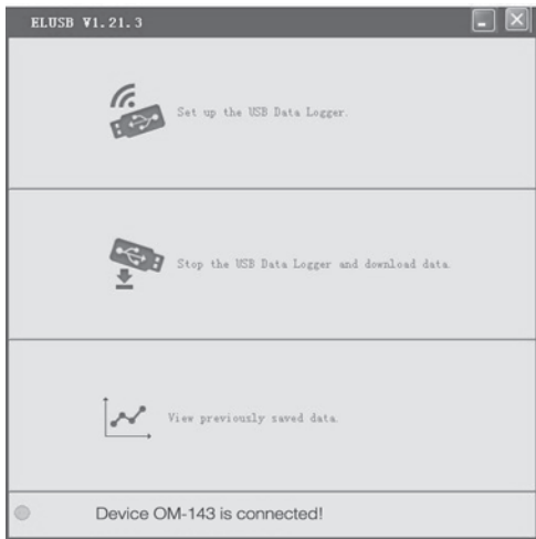
Fig. 2. The three options made available by plugging the OM-143 into a USB port
