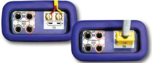
Simulating or reading RTDs uses copper wire.
