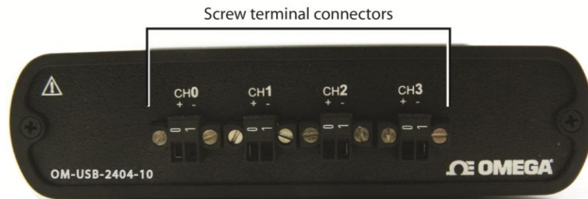
Figure 2. Front panel (Screw terminal connections)
