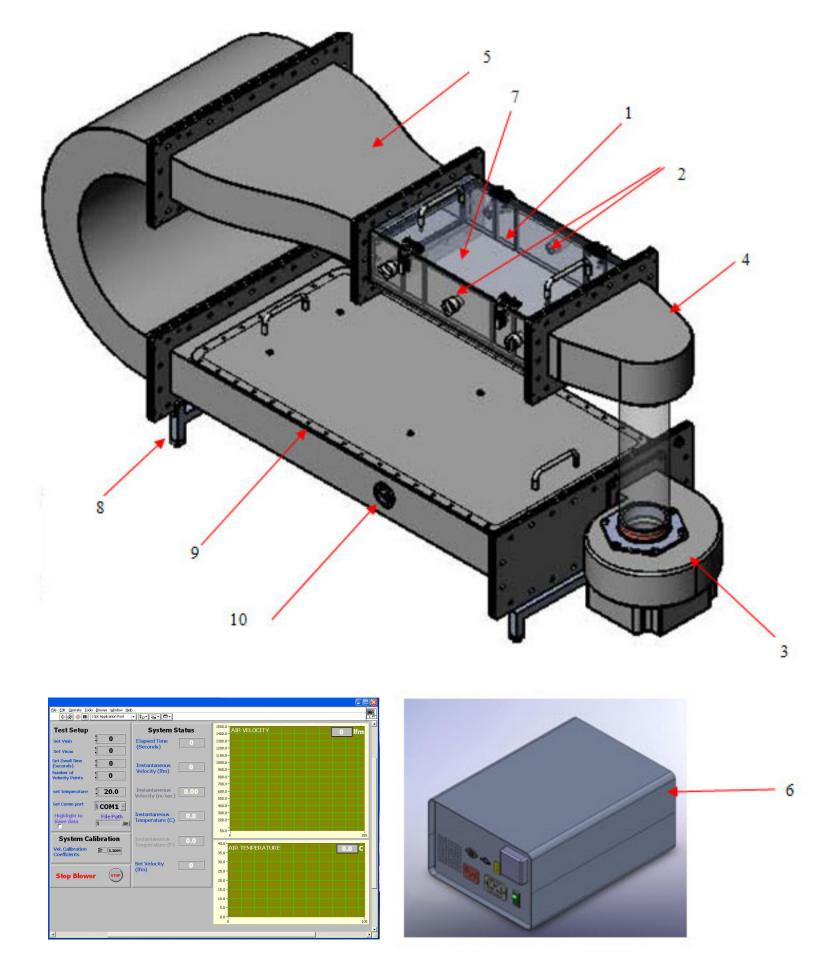
Figure 1: The WT-3067 System Components
