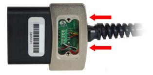
5. Reinstall the cover and tighten the two Phillips screws.
