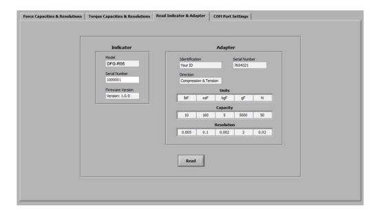
Use this screen to view information about the sensor and indicator. Click **Read** to view the indicator model number, serial number, and firmware version. The sensor's identification number, serial number, direction(s), capacities, and resolutions are also visible.
