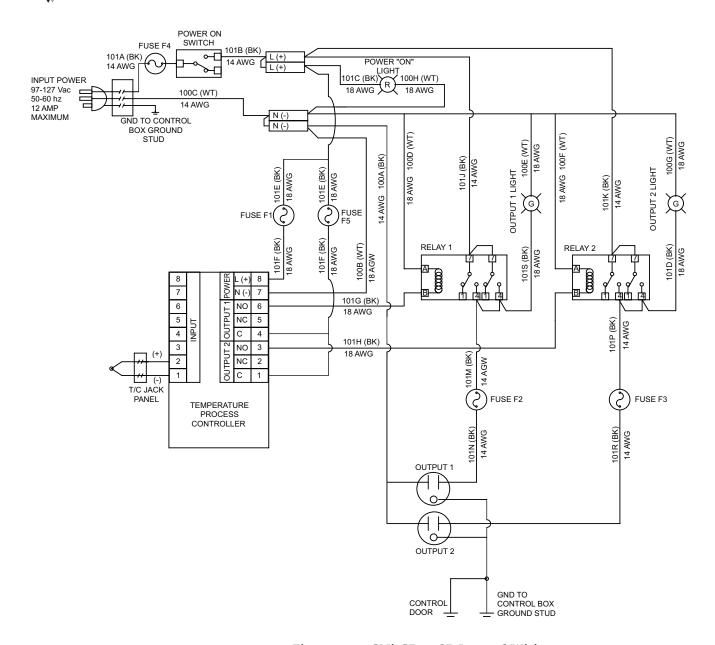
Figure 3-10. CNi-CB120SB Internal Wiring
