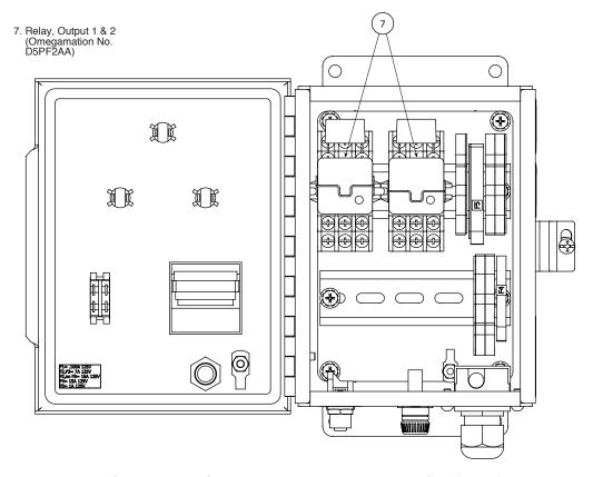
Figure 2-7. CNi-CB120SB Components, Front View (Open)
