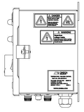
Figure 2-2. CNi-CB120SB Labels, Right View
