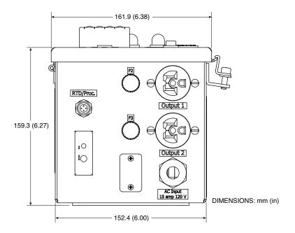
Figure 2-5. CNi-CB120SB Mounting Dimensions, Bottom View
