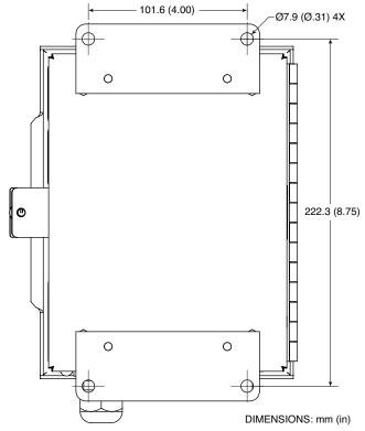
Figure 2-3. CNi-CB120SB Mounting Dimensions, Rear View
