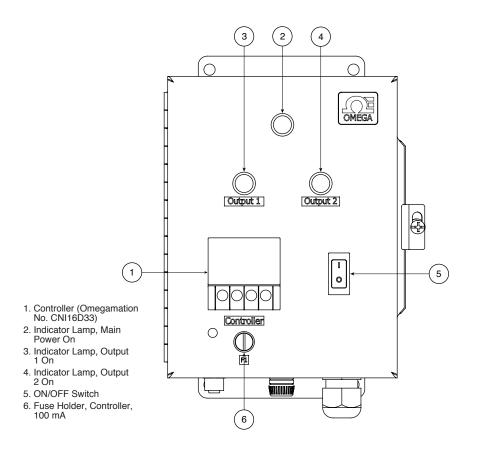
Figure 2-6. CNi-CB120SB Components, Front View (Closed)
