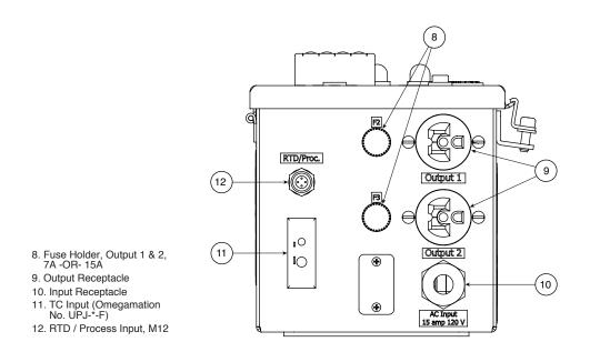
Figure 2-8. CNi-CB120SB Components, Bottom View
