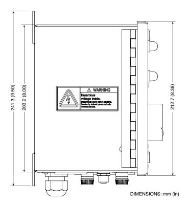
Figure 2-4. CNi-CB120SB Mounting Dimensions, Side View
