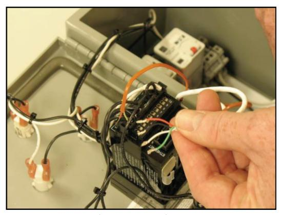
Figure 3-4. Remove Wire Nut
