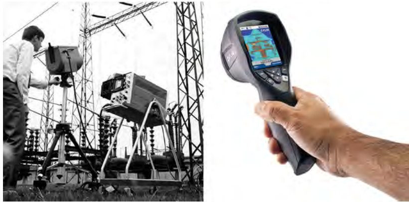
Figure 13.2 LEFT: Thermovision Model 661 from 1969. The camera weighed approximately 25 kg (55 lb.), the oscilloscope 20 kg (44 lb.), and the tripod 15 kg (33 lb.). The operator also needed a 220 VAC generator set, and a 10 L (2.6 US gallon) jar with liquid nitrogen. To the left of the oscilloscope the Polaroid attachment (6 kg/13 lb.) can be seen. RIGHT: Flir i7 from 2012. Weight: 0.34 kg (0.75 lb.), including the battery.
