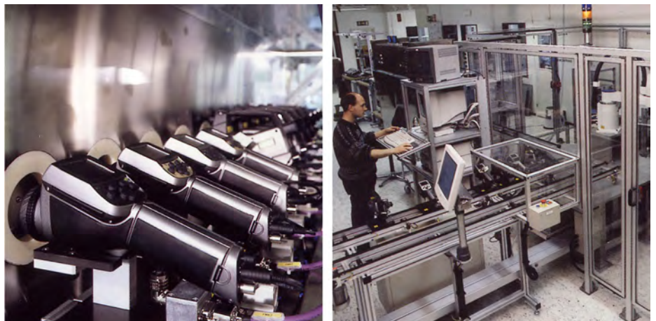
Figure 13.5 LEFT: Testing of infrared cameras in the climatic chamber; RIGHT: Robot used for camera testing and calibration
