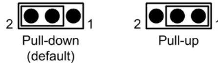
Figure 9. W1 jumper configurations
