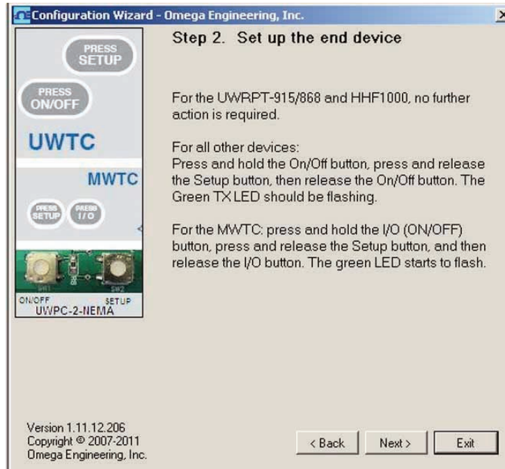
Figure 5-6. Utility Program - Setup Transmitter Screen
