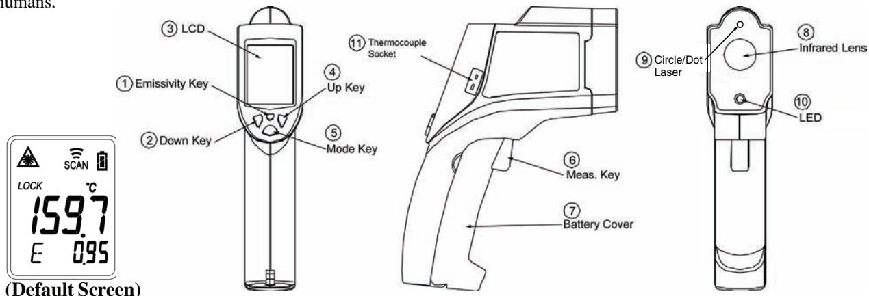
Simply aim the thermometer at the measure target with Lens (8) and press Meas. key (6) to display the surface temperature. The Distance:Spot is 35:1. The laser circle/dot points are the reference for the target spot size. Please make sure the target area is within the field of view.
