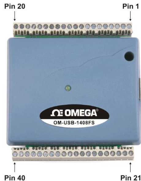
Figure 4. OM-USB-1408FS Screw terminal pin numbers
