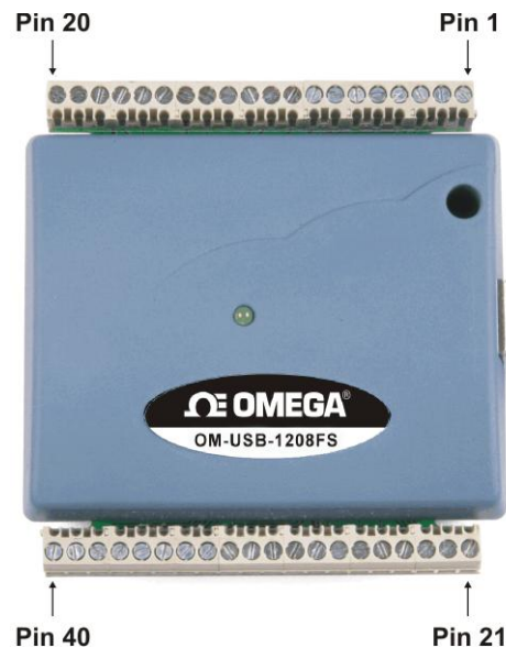
Figure 4. OM-USB-1208FS Screw terminal pin numbers
