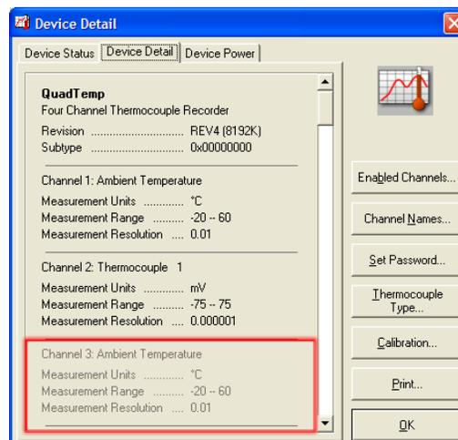
Notice that disabled thermocouple and ambient channels appear greyed-out on the Device Detail screen.
