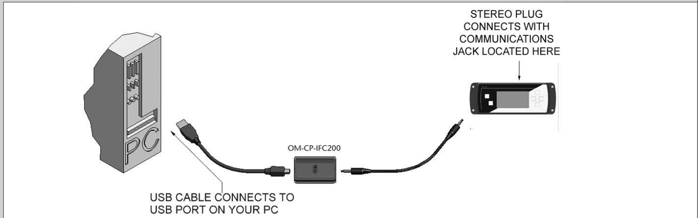
Fully insert the male connector of the OM-CP-IFC200 interface cable into the female receptacle of the data logger. Fully insert the female USB connector into the USB. *(Please see the OMEGA Datalogger Software manual for further information)*
