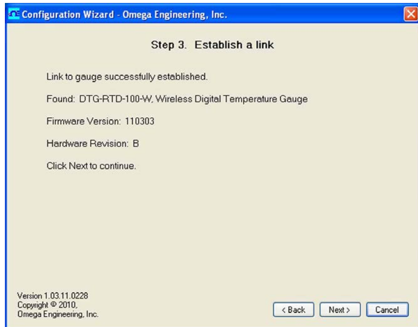
Figure 3-13. Utility Program - Establish Link Screen
