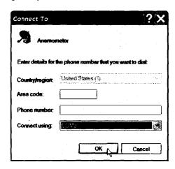
In the next window, select the port settings as shown below and click OK. (The Serial Port settings are also listed at the end of this section).
