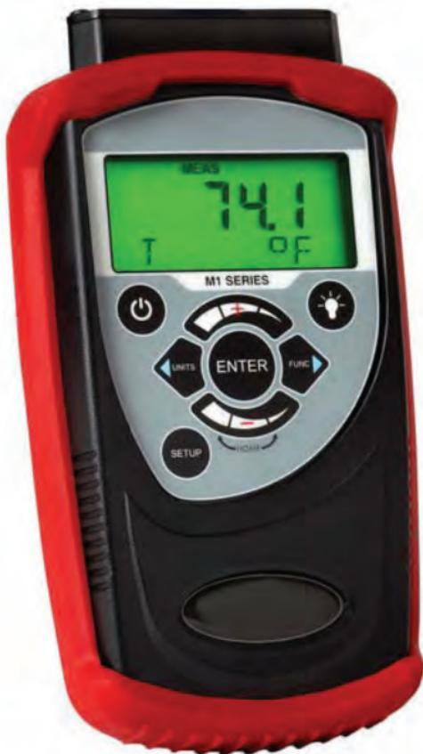
The T/C calibrator is a handheld unit for thermocouple (T/C) measurement or simulation. Eight T/C types are supported referencing NIST175 and ITS90 standards. Temperature can be displayed in selectable engineering units of °C, °F, °R, K and mV.
