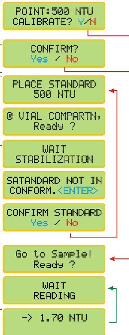
**Attention: for TURBIDITY, this instrument MUST BE calibrated using Formazine Standard and cannot be calibrated using Polymers!!!**
