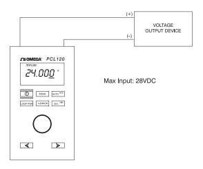
Figure 6 - Measuring 0 to 28 VDC
