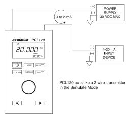
Figure 4 - Simulating 4 to 20 mA
