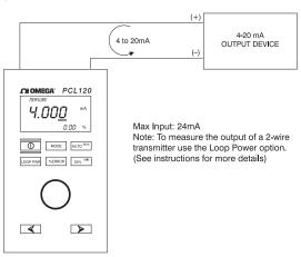
Figure 5 - Measuring 4 to 20 mA
