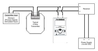
The CL531 can read loop currents from 0-24 mA. The CL531 limits current in read mode to 25mA to protect the devices in the loop from over voltage or over current conditions.
