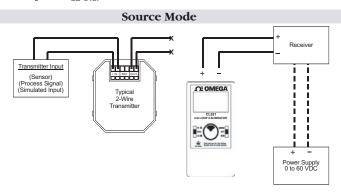
Source mode uses internal power to supply current from 0.00-24.00 mA into as much as  $1200\Omega$  until the end of battery life. The calibrator Graph will flash if connected improperly. The three-position EZ-Check switch provides instant preset 4mA at zero, 12mA at mid range and 20mA at full scale outputs. The output is adjusted in 0.01 or 0.10 mA increments (0.1 or 1.0) % display units with the EZ-Dial knob.
