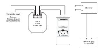
The CL531 supplies 15Volts or 24 Volts to the transmitter and displays the output in mA or % on the CL531 display. In read mode press the EZ-Dial™ Knob twice to get into the feature options. Then press the EZ-Dial™ Knob to select mA PWR - M. Then turn EZ-Dial™ Knob to select power range (15V or 24V). The EZ-Check switch and EZ-Dial knob allow rapid and fine control of loop current.
