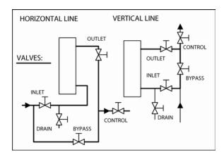
⚠ Valves must be closed prior to installation and opened gradually after all connections are carefully inspected. A leak test is highly recommended especially when hazardous fluids are involved.
