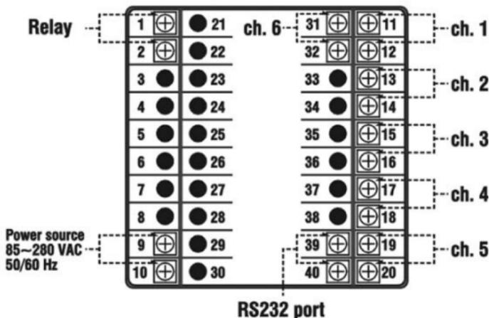
**All of the channel labels :** Each channel requires a positive and negative wire. This picture shows which channels represent which input terminals and if they are negative or positive.
