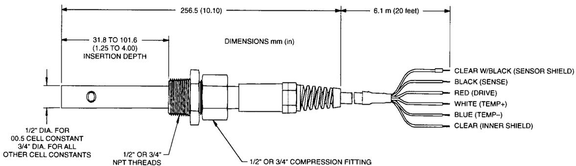
Figure 2-1. General Dimensions and Cable Wire Details
