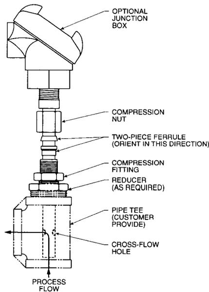
**Figure 2-3. Compression Fitting Parts Arrangement For Insertion Mounting**
