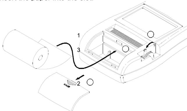
4. Press **FEED** multiple of times to load the paper into printer.
