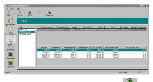
To perform a new test procedure, you have to select the Tag and then to press the Buntest button. The following window will be displayed:
