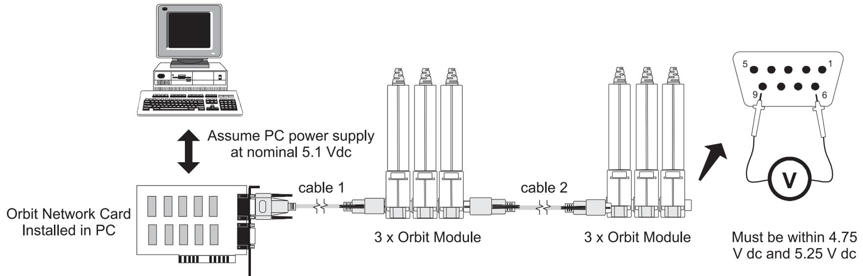
$$\begin{aligned} \text{Volt drop total in mV} &= \text{cable 1 + module (3 off) + cable 2 + module (3 off)} \\ &= (15.2 \times 6) + 0.04(6+5+4+3+2+1) + (15.2 \times 3) + 0.04(3+2+1) \\ &= 138 \text{ mV} \\ \text{Then approximate voltage at end of network} &= \text{nominal supply voltage - calculated volt drop} \\ &= 5.1 - 0.138 \\ &= 4.96 \text{ V} \end{aligned}$$
