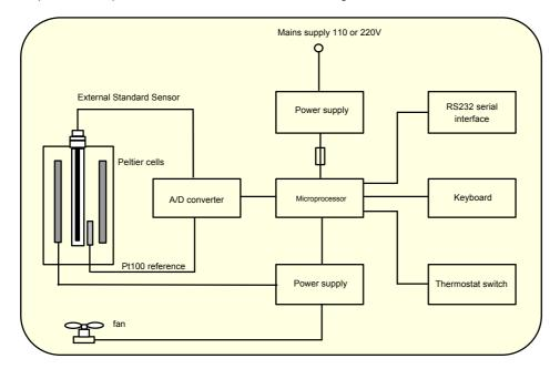
The instrument functional blocks of the instrument are as it follows:
