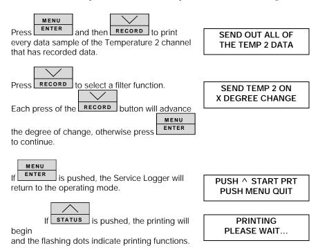
When the Service Logger is finished printing it will return to the Operating Mode.
