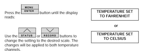
When the button is pressed twice more (to cycle through the remaining functions), the temperature scale setting will be saved into memory, and the Service Logger will return to the operating mode. Otherwise the unit will return to the operating mode after approximately 1 minute and changes will be saved into memory.
