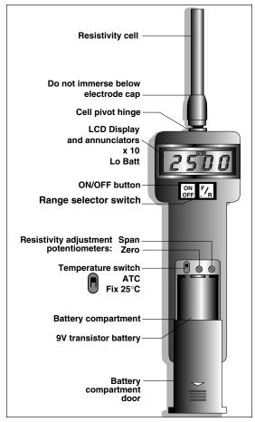
Figure 1. Parts of the Meter
