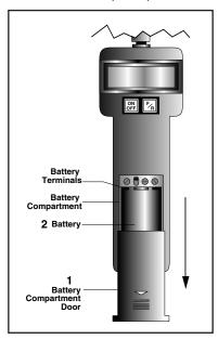
Figure 2. Installing the Battery
