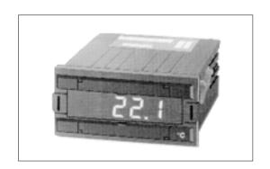
DC INSTRUMENT 3  $\frac{1}{2}$  DIGITS, FOR SIGNAL INPUT IN Vdc UP TO 200 Vdc, IN TWO RANGES SELECTABLE ON THE SIGNAL CONDITIONER BY PLUG-IN JUMPERS. ALLOWS THE READING TO BE DISPLAYED IN ENGINEERING UNITS, USING THE TRIMMERS AND SELECTABLE RANGES FOR SPAN AND OFFSET (see fig.3).
