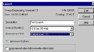
To start the RD-TEMP, modify the settings as desired, then select **Start**. Disconnect your RD-TEMP after launching. The RD-TEMP's LED will blink once with each measurement. For long periods of use, the LED will blink weakly every two seconds between measurements.
