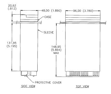
Figure 21-3. Meter Dimensions with Standard Bezel
