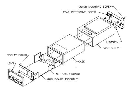
Figure 2-2. Exploded View of Meter with Optional Housing
