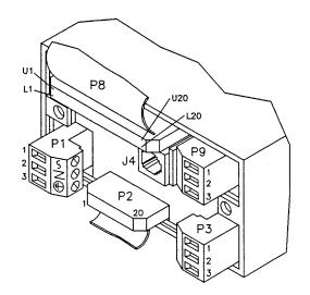
Figure 7-2. Rear View of Meter with BCD and Serial Communication
