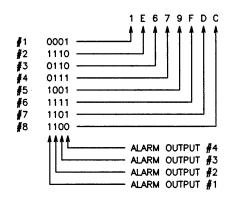
The 1's represent an ON output and the 0's an OFF output. One pattern group can hold eight of these switch patterns. One switch pattern is stored inside one nibble of information. This totals eight bytes. These pattern groups are only stored in non-volatile memory, therefore you may use only the R,W commands. Refer to Table 15-5 for more information on Hex conversions.
