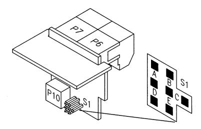
Figure 17-1. Dual Relay Output Board
