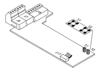
Figure 18-1. 4-Relay Board Jumper Locations
