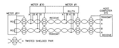
Figure 15-6. Multi-Point Full-Duplex RS-485 Connection
