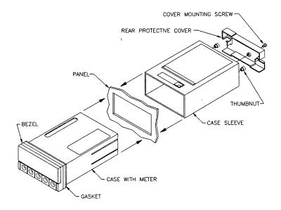
Figure 21-2. Panel Mount Assembly with Standard Bezel
