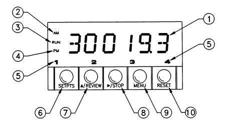
Figure 2-4. Front-Panel Display and Buttons
