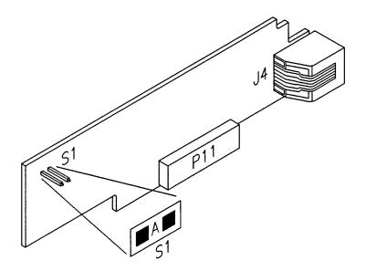
Figure 15-1. RS-232 Serial Communications Board
