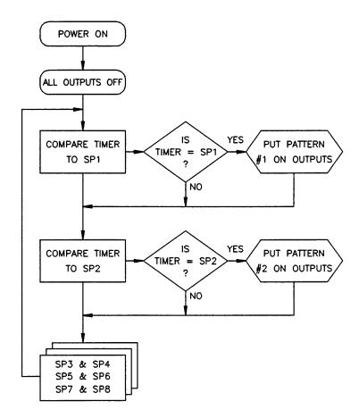
Figure 14-7. INDPAT Mode Flowchart
