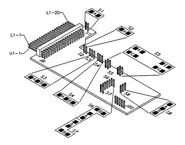
Figure 16-1. BCD Board Jumper Locations
