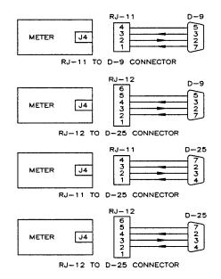
Figure 15-3. 4-Wire RS-232 Connections
