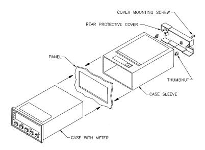
Figure 21-4. Panel Mount Assembly with Optional Housing
