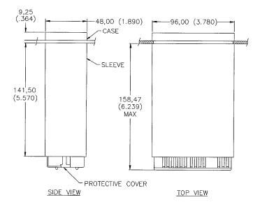
Figure 21-5. Meter Dimensions with Optional Housing
