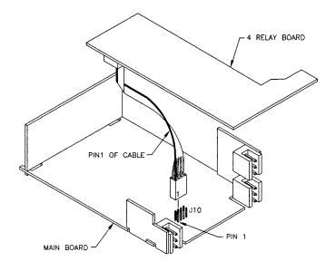
Figure 18-2. 4-Relay Board Installation
