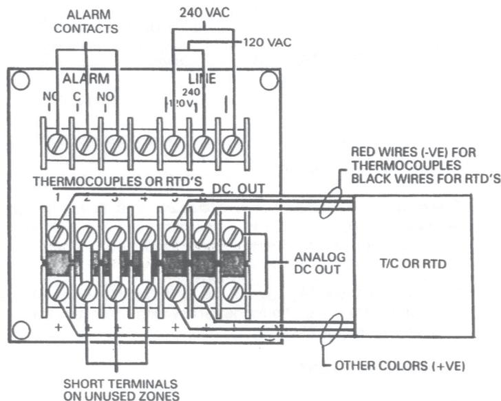
Figure 2-2. Wiring Diagram
