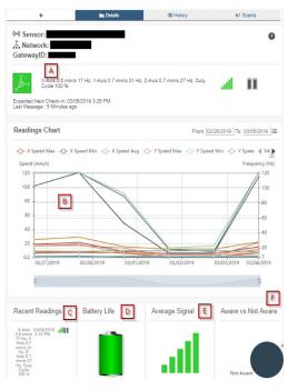
A. The sensor overview section will be above every page. This will consistently display the present reading, signal strength, battery level, and status.
